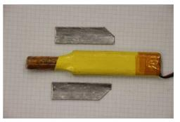
Balance the model for the first time. Depending on the desired location of the centre of gravity (see below), 20-100g of lead is required in the nose. The weight is positioned in front of or beside the battery. Weigh the required amount of lead.
