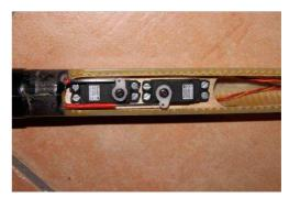
The length of the servo horn is 8mm. Position the servos in longitudinal direction so that both rods have sufficient space to move up to their entry point into the fuselage. Imagine that the clevis joint is screwed on to the carbon rods (see below). Apart from this, the servo board shall of course be as far up front as receiver and battery permit.
