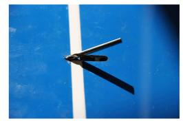
and underlay the tension pin/Achsstift with 1.5mm vis-à-vis the wing contour (see picture with white surface)
