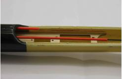
When everything has been tested, fit the servo board in, using UHU endfest. Roughen up the surface well by sanding the fuselage as the bonding of servo board and fuselage contributes considerably to the stability of the front part of the fuselage. Also ensure that the servo board is securely fitted in the back part between the wings.
