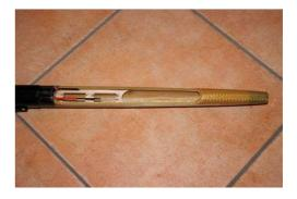
It is also important that the niche between servo board and fuselage frame is not filled with too much glue, given that otherwise there would not be sufficient space left for the wing cables. It would be best to run along the edge of the niche with a spatula to clear it of the glue. A triangle measuring approximately 3mm edge length should remain as adhesive beading.
